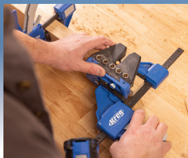
Designed for use with trigger style clamps for improved accuracy and stability
