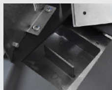
Glue Assembly Has a recycle system that allows excess glue to flow back into the gluepot
