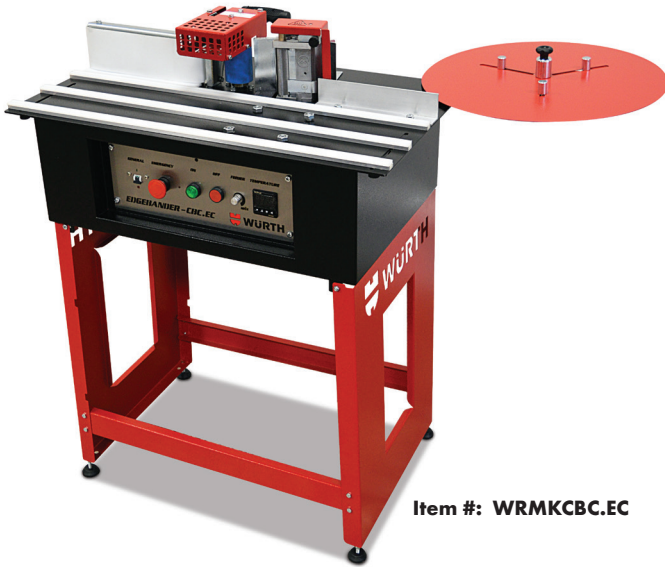
Large Plate Support Fits a 20" roll of edge-banding tape
