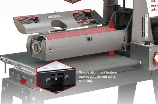
Fast Lever makes it easy to change alignment settings for narrow and wide stock.
