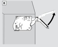
Carefully remove the transport tab.
