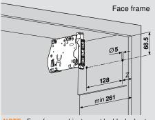
**NOTE:** Face frame cabinets must be blocked out flush with the frame.
