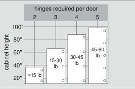
NOTE: The distance between the top and bottom hinges must be greater than the width of the door
