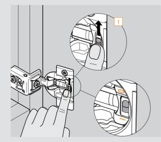
Door must be closed once for the deactivation to be complete. To reactivate, move switch back to the original position "I".
