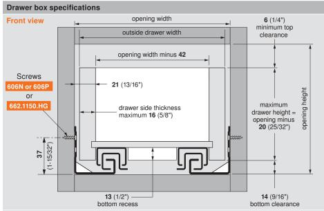
**NOTE:** Drawer side material thickness may vary. Accurate measurement of drawer side material thickness should be used when calculating outside drawer width using the table below. Inside drawer width **must** equal opening width minus **42** (1-21/32") for TANDEM to align and function optimally.
