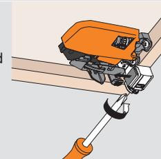
Turning the adjustment screw allows for up to a +2.5 (3/32") out adjustment
