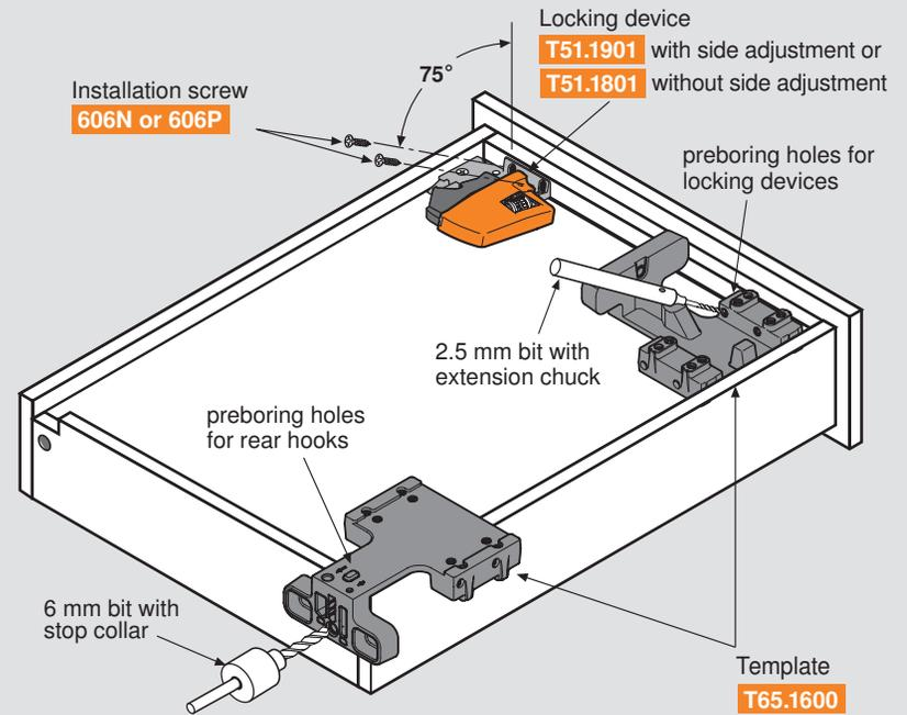
**NOTE:** Use of the T65.1600 template is essential for accurate location and angle of pre-bored locking device holes and accurate boring for rear hook holes
