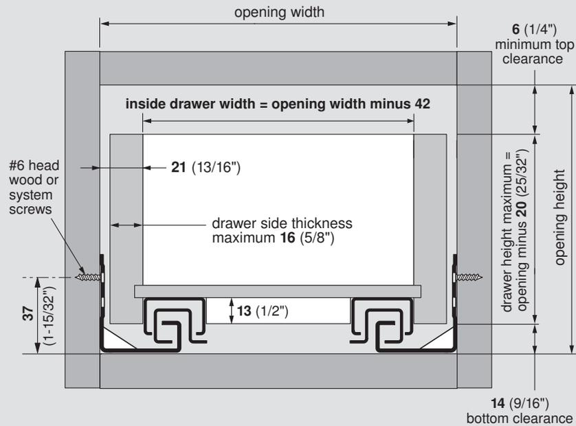
**NOTE:** Because material thickness may vary, the inside drawer width must equal opening width minus 42 for TANDEM to align and function properly
