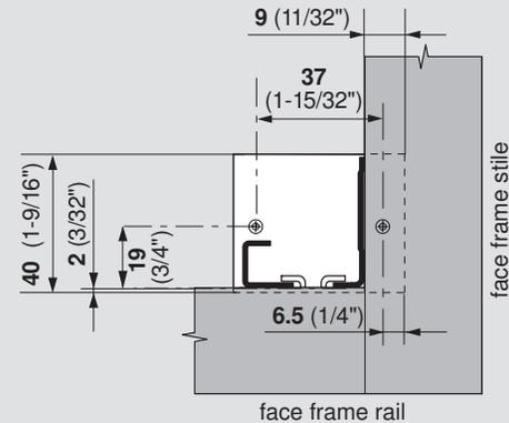
**NOTE:** Use at least three 606N or 606P installation screws for 295.3750.01 or 295.3700.2x
