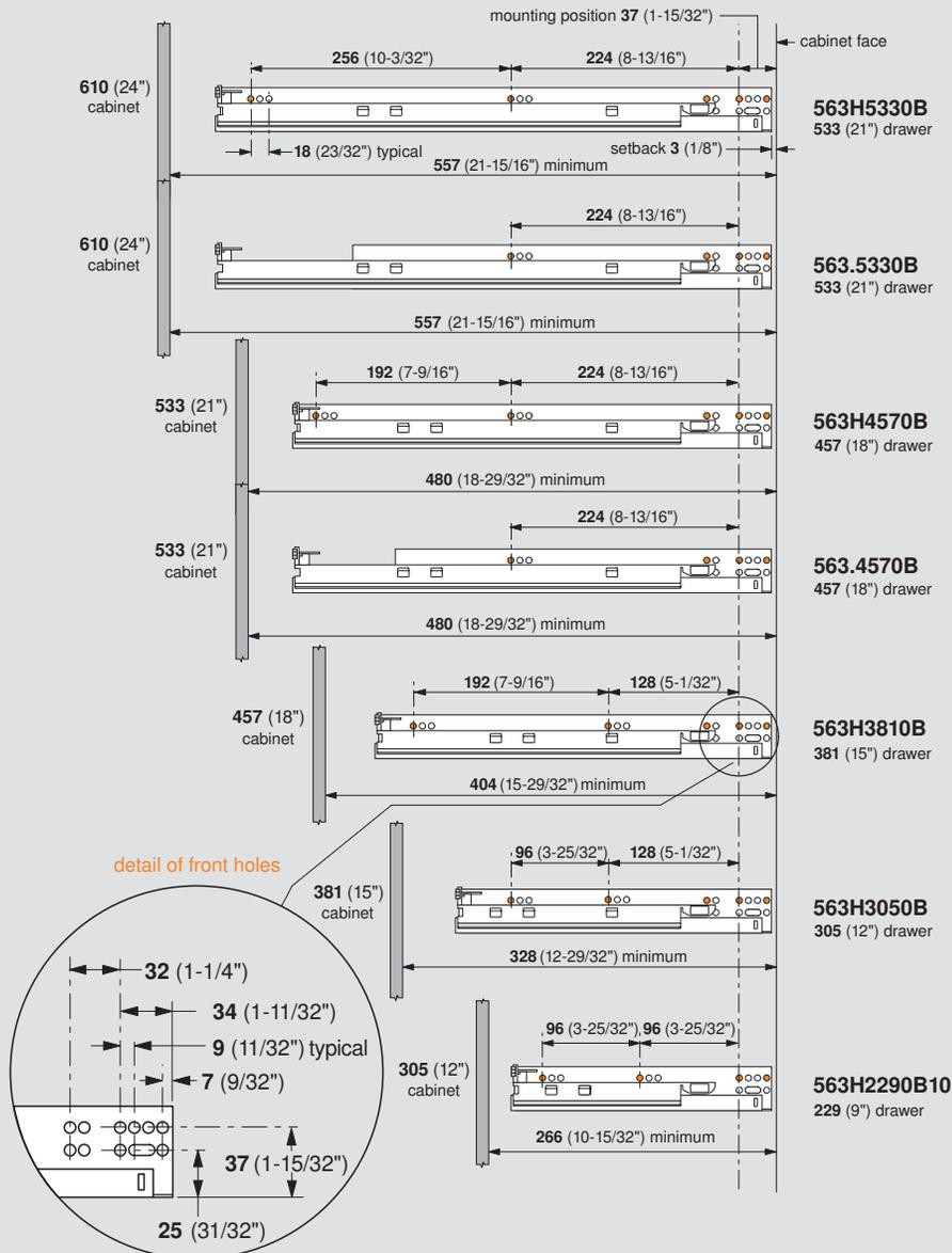
**NOTE:** Orange dots indicate screw locations required to meet specified load capacities
