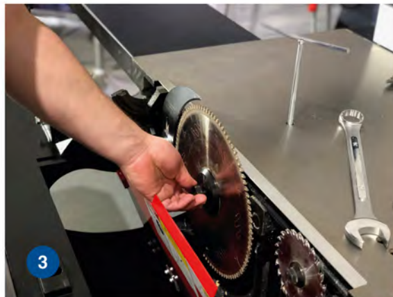
Fig. 1 and 2: Hold it down from the top and loosen side nut clockwise. Fig. 3 Tighten the nut.
