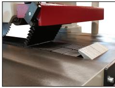
ANTI-KICKBACK FINGERS (3) sets of anti-kickback fingers (2) top and (1) set in the table for safe operation.
