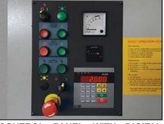
CONTROL PANEL WITH DIGITAL THICKNESS ADJUSTMENT
