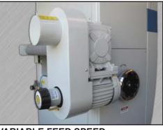
**VARIABLE FEED SPEED** Variable feed speed allows the operator to choose the correct sanding speed for various sanding applications, belt grits, wood species, and desired results.
