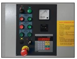
CONTROL PANEL WITH DIGITAL THICKNESS ADJUSTMENT - Centrally located control panel for convenient operator access. Includes digital motorized thickness adjustment to 3-decimal places in Inch & 2-decimals in MM. Also emergency stop button, ammeter for load monitoring, and
