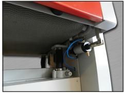
CONVEYOR BELT TRACKING & HEIGHT ADJUSTMENT SCREWS
