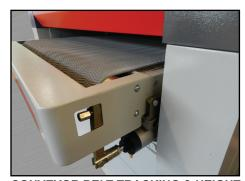
CONVEYOR BELT TRACKING & HEIGHT ADJUSTMENT SCREWS
