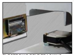
**ELECTRONIC BELT TRACKING** Electronic send & receive sensor precisely detects the sanding belt for most reliable belt tracking. Machine is also equipped with belt overrun limit switches for added safety.
