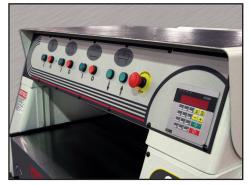
DIGITAL THICKNESS CONTROL Equipped with a digital thickness control which can be programmed in Inch of Metric. To 3-decimal places in inches and 2-decimal places in Millimeters.
