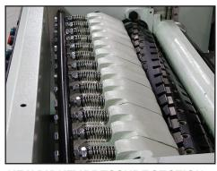
**HEAVY DUTY PRESSURE SECTION**Sectional chipbreakers and section infeed pressure roller for positive feeding of material. Rubber covered outfeed roller. Anti-kickback fingers are installed for added safety
