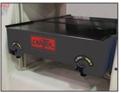
PRECISE BED ROLL ADJUSTMENT Convenient bed roll adjustment on the front of the feed table allows for precise setting of the powered bed rolls for the best possible feeding results
