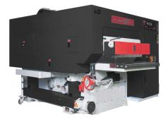
**OPTIONAL CE GUARD** Optional fully enclosed guard cover with limit switches on doors to CE standard.
