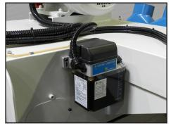
**AUTOMATIC LUBRICATION** Conveyor system is constantly lubricated by an electronic oiler ensuring maximum life with minimum wear
