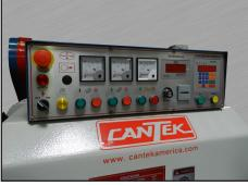
**CONTROL PANEL** Convenient operator control panel with digital thickness control (mm/inch), individual amp meters for cutterheads and feed, digital speed display, hour meter, and emergency shut off. Rotates 90°
