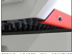
**SPRING LOADED PIN CONVEYOR SYSTEM** Pins have up to 3/4" travel and conform to each individual work piece. Designed to pass material over the bottom jointing head
