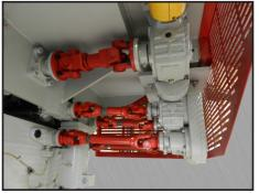
**CARDAN SHAFT FEED DRIVE** The flexible cardan drive provides maximum feeding power with higher capacity feed rates
