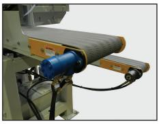
**POWERFUL HYDRAULIC FEED DRIVE**Both main and return conveyors are hydraulically driven for a powerful and consistent feeding operation.
