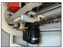
**DOVETAIL TEMPLATES & MOTOR** Equipped with (4) dovetail templates for producing a range of dovetail joints. Powerful 1HP dovetail spindle motor.
