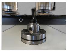
PRECISION SPINDLE ASSEMBLY 18500 RPM precision spindle ensures a clean cut. An eccentric single flute cutter can be adjusted in the chuck to loosen or tighten the joint.
