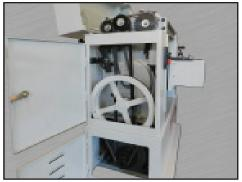
FEED MECHANISM & MACHINE FRAME Equipped with two feed speeds which are easily accessed through the side doors. A powerful chain feed system provide superior feeding results. The machine frame/table is mostly cast iron, with a heavy duty welded steel body.
