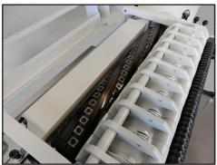
SPIRAL INSERT KNIFE CUTTERHEAD The spiral insert knife cutterhead provides a smooth finish with a quiet cutting operation. 4-sided solid carbide insert knives can be easily rotated for a new sharp cutting surface.
