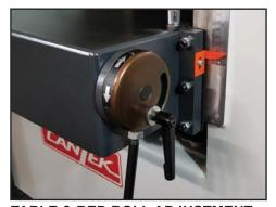
TABLE & BED ROLL ADJUSTMENT The idle bed rolls are conveniently adjusted from the front of the table. The eccentric cam allows you to raise and lower the bed rollers and can be locked in place for optimum feeding results on both rough and smooth material.
