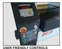
Equipped with digital thickness control with dual INCH/Metric display. The digital control
