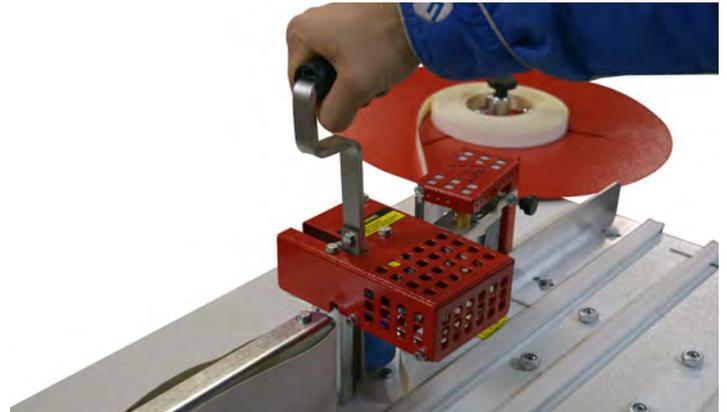
According to the first tests you will find an ideal amount of glue that must pass the panel. In case you notice that the tape is easily released from the wood, the cause may be lack of glue. Or if not, there may be glue excess, with glue excess on the sides of the tape. To adjust the glue thickness, do the following:
