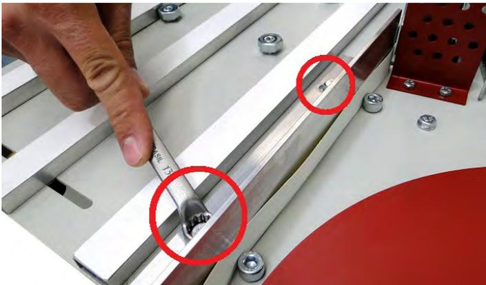
4. Insert the sample piece of tape behind the aluminum guide, between the guide and the Allen screws, as seen in the figure above.
