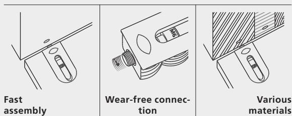
Cabineo 8 M6 is a one-piece cabinet connector which can be used with all CNC machines because only surface machining is required. The connector is ideal when joining wood composites with materials such as aluminium, steel or compact laminate.
