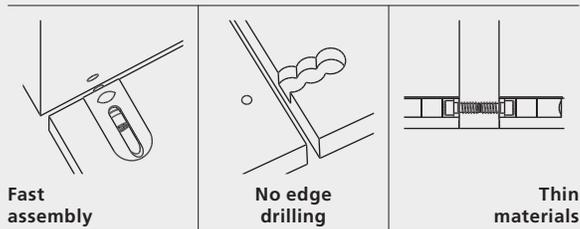
Cabineo 8 is a one-piece cabinet connector which can be used with all CNC machines because only surface machining is required. The Cabineo is installed in the board either in the workshop or on site. The pre-assembled screw in the connector is screwed into the 5 mm hole of the second workpiece using a cordless drill. Cabineo impresses with its time-saving processing and assembly as well as the high clamping force which leads to stable connections without the need for additional dowels.
