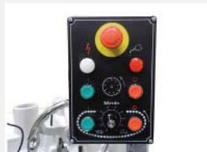
Eye level control with emergency stop button and low oil warning light
