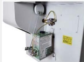
Automatic mechanical lubricator ensures long chain and track life
