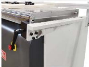
Side fences can be safely and easily folded away when not in use
