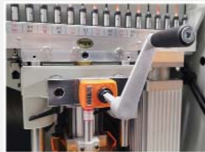
Boring height is conveniently and accurately adjusted with a mechanical counter
