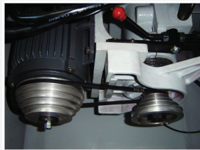
Powerful 7.5 HP motor with 5 spindle speeds
