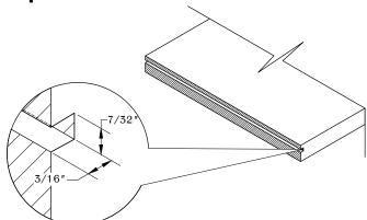
Rout slot for BR on desired surface.
