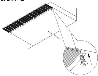
Screw BR strip onto desired location. Note: Screws not included.
