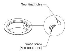
Use (2) Wood screws through the BRV1 mounting holes to secure on to the table top.
