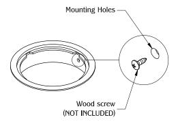
Use (2) Wood screws through the BRV2 mounting holes to secure on to the table top.
