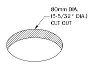
Make a cut out on the desired surface. (<u>Note</u>: We do not recommend cutting before receiving part or part sample.)
