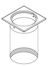
Install BRV2/SQ into the cut out and be sure it is fully leveled onto work surface.
