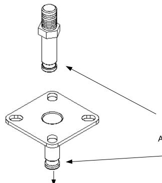
Apply grease to the bottom of top plate or stem.
