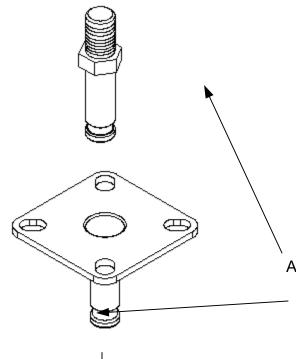
Apply grease to the bottom of top plate or stem.
