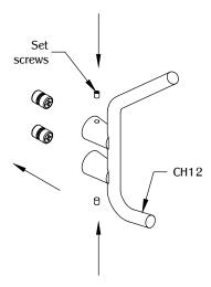
Align the base of the part to the mounting sleeve. Use the hex key to secure the the assembly with (2) set screws from the top and bottom of the base.
