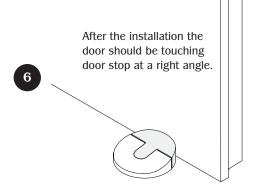
Prior to any installation please consider the weight of the door, impact angle of the door against the door stop, height of the lower door corner and the type of floor. Depending on these factors different door stops or installation hardware should be considered.
