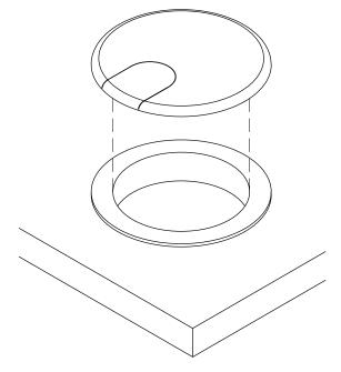
Install EDP1 into the cut out and be sure it is fully leveled onto worksurface.
