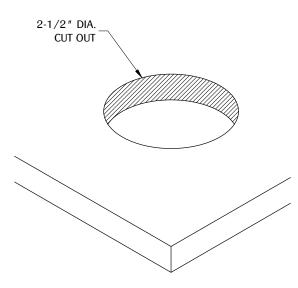
Make a cut out on the desired surface. (<u>Note:</u> We do not recommend cutting before receiving part or part sample.)
