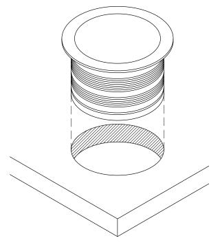
Install EDPAD1 into the cut out and be sure it is fully leveled onto worksurface.
