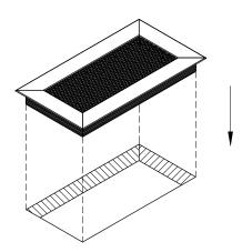
Install the unit into the cut out and make sure it is fully leveled onto the surface. (Note: Apply adhesive for a more secure and permanent installation.)
