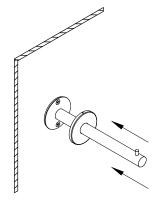
SLIDE COVER PLATE OVER BACK PLATE TO CONCEAL MOUNTING HARDWARE.
