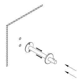
PLACE BACK PLATE OF HNGH2 OVER HOLES AND APPLY WOOD SCREWS.
