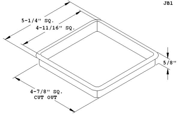
All dimensions have a 1/32" tolerance unless otherwise specified. We do not recommend drilling or cutting any holes before receiving a product or a product sample.
