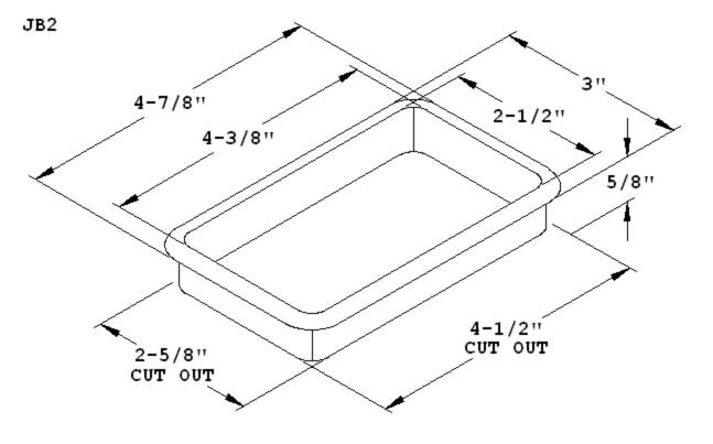
All dimensions have a 1/32" tolerance unless otherwise specified. We do not recommend drilling or cutting any holes before receiving a product or a product sample.
