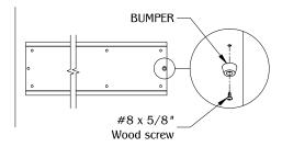
Mount the track on the underside of the work surface using (8) #8 wood screws.
