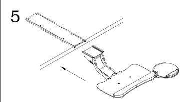
Slide the KP8 tray and mechanism into the mounted track.
