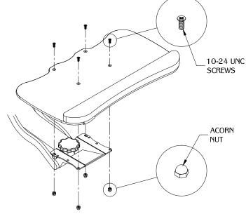
Secure the mechanism to the tray with (4) 10-24 countersunk screws and (4) acorn nuts.
