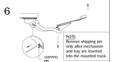
Tip front of the KP8 tray up and begin to lower mechanism to relieve pressure on the shipping pin. Pull out the shipping pin.
