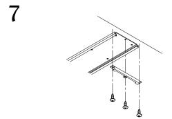
Slide the mechanism back to the bumper. Install the track guard at the front end of the track using (3) #8 wood screws.
