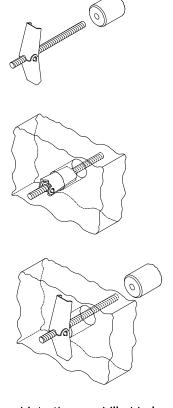
Step 2: Thread the wing onto the appropriate threaded hardware and place the wing end into the pre-drilled hole in the wall surface. DO NOT let go of the threaded end as it will fall behind wall surface.
