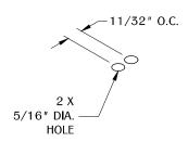
Drill two 5/16" diameter holes on the desired work surface for the positioning pin and the threaded screw.
