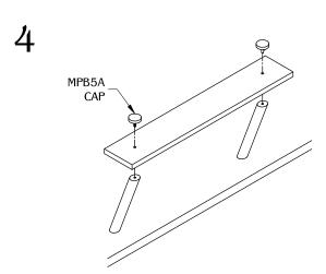
Align the drilled holes of the shelf to match the MPB5A barrel. Secure the shelf with MPB5A cap.
