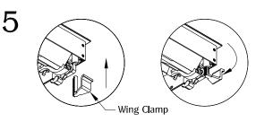
Secure unit by turning bottom wing clamp.
