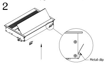
Place metal clips near the ends of the back of the unit. (NOTE: Metal clips are for use in hard surface material only as an optional mounting means.)
