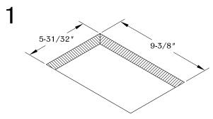
Determine the position and location of the unit on the work surface. Cut the hole at 9-3/8" X 5-31/32". Place and allow enough clearance for unit operation. DO NOT place unit where the cable is strained or trapped.
