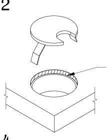
ADD ADHESIVE AND INSERT SLEEVE ALLOWING A 1/8" SPACE FOR CAP TO FIT FLUSH WITH SURFACE
