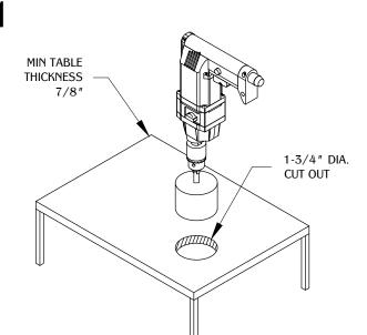
Make a cut out on the desired surface. (Note: We do not recommend cutting before receiving part or part sample.)
