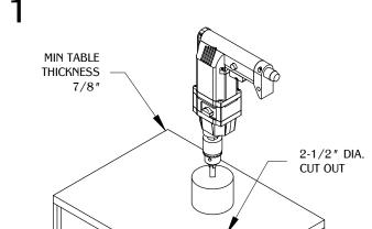
Make a cut out on the desired surface. (<u>Note</u>: We do not recommend cutting before receiving part or part sample.)
