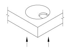
NOTE: IN ORDER TO REMOVE STEEL CAP YOU WOULD NEED TO PUSH FROM THE BOTTOM UP.
