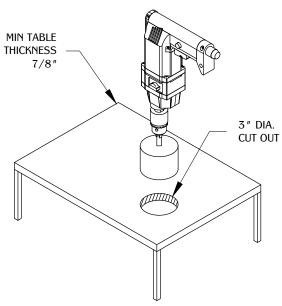
Make a cut out on the desired surface. (Note: We do not recommend cutting before receiving part or part sample.)
