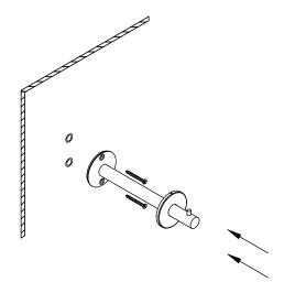
PLACE BACK PLATE OF HNGH1 OVER HOLES AND APPLY WOOD SCREWS.
