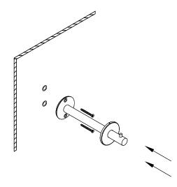
PLACE BACK PLATE OF HNGH2 OVER HOLES AND APPLY WOOD SCREWS.
