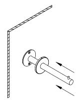
SLIDE COVER PLATE OVER BACK PLATE TO CONCEAL MOUNTING HARDWARE.
