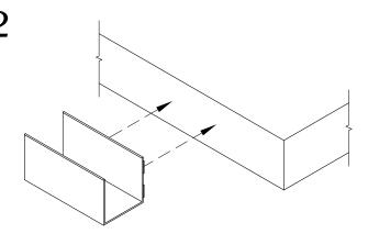
Apply adhesive or double-sided tape to the back of the WM9. If purchased with double-sided tape pre-installed, proceed to step 2.
