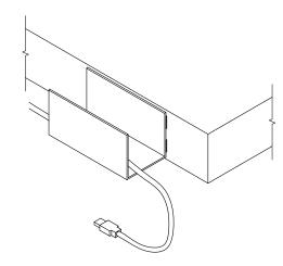
Apply pressure to the WM9 when placing against the work surface until it is held into position by the adhesive.
